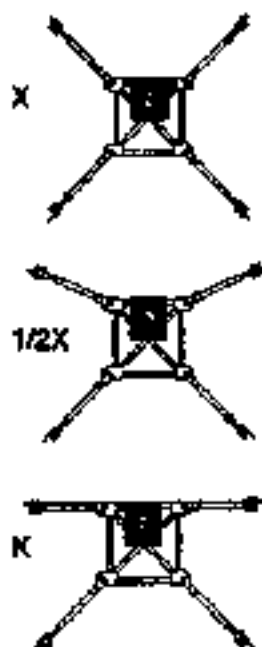
Fig. 3-40) Extending legs position
